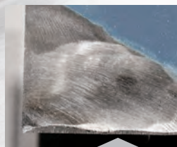
Surface finishing by grinding
